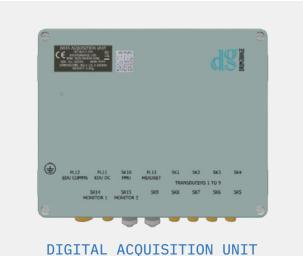
HULL VIBRATION MONITORING EQUIPMENT
